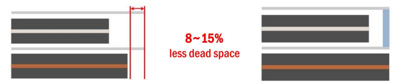
By minimizing the dead space by extra separator, we can achieve higher energy density than the competitors' technology with the same dimension and same material.
